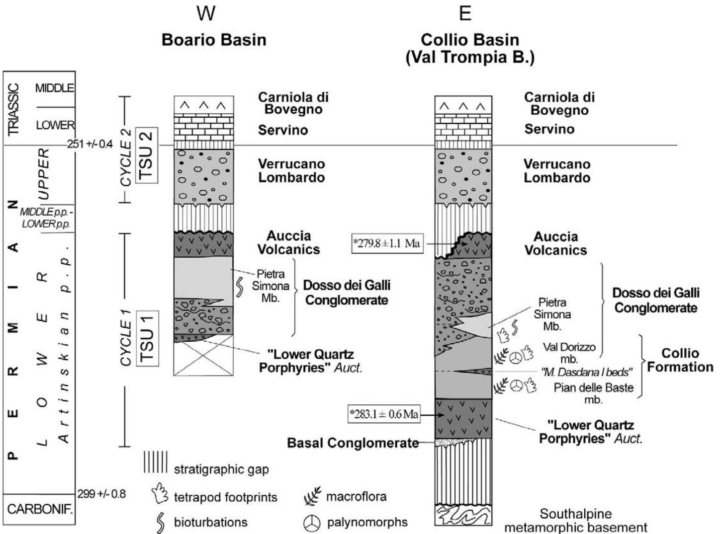
Fig. 2 – Synthetic stratigraphic columns in central Southern Alps, from the typical Lower Permian Collio Basin (E), in the Val Dasdana-Passo Maniva area, and the close small Boario Basin (W), in the lower Val Camonica. Vertical distances are not time- or thickness-related. Geologic time scale from Gradstein *et al.* (2004a).
